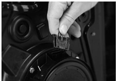
The IC 165VW Woofer connectors are the same used by Volkswagen® standard.
